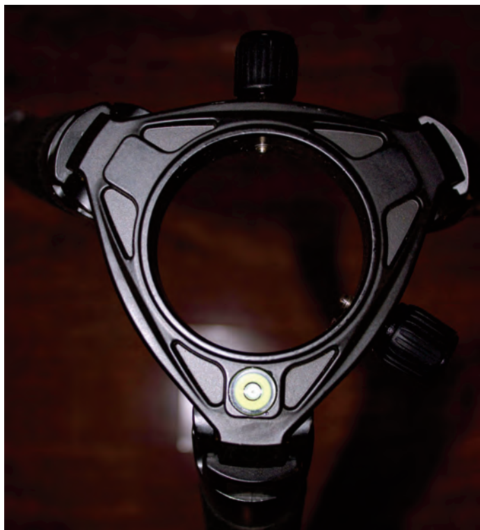
Image 2 – The tripod has a bubble level and two thumb-screws that securely hold the telescope in place.
