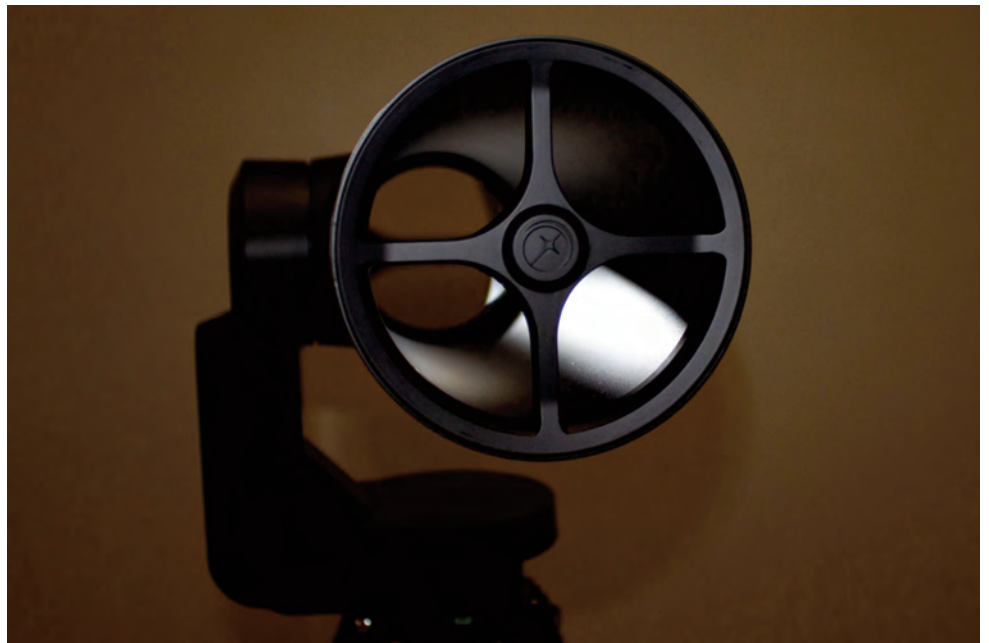
Image 5 – This view shows the one-arm fork mount and the inside of the OTA.
